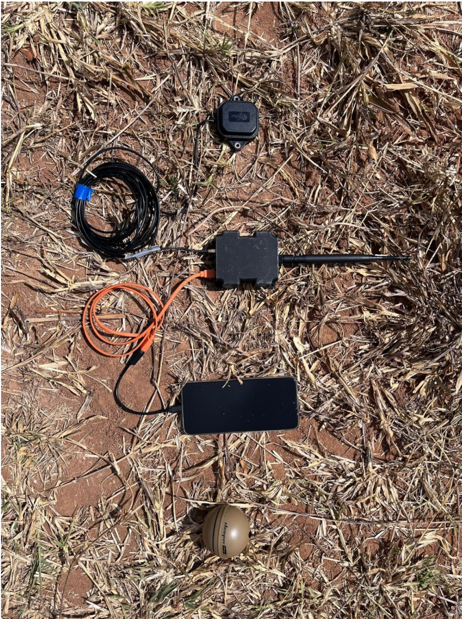
Figure 2.1: From top to bottom: GNSS antenna, GNSS chipset (ublox ZED-F9P on an arduSimple breakout board), Android smartphone and a Deeper Chirps 2+ fish finder. Cabling is for connecting the GNSS antenna to chipset and reading GNSS data on the smartphone.
