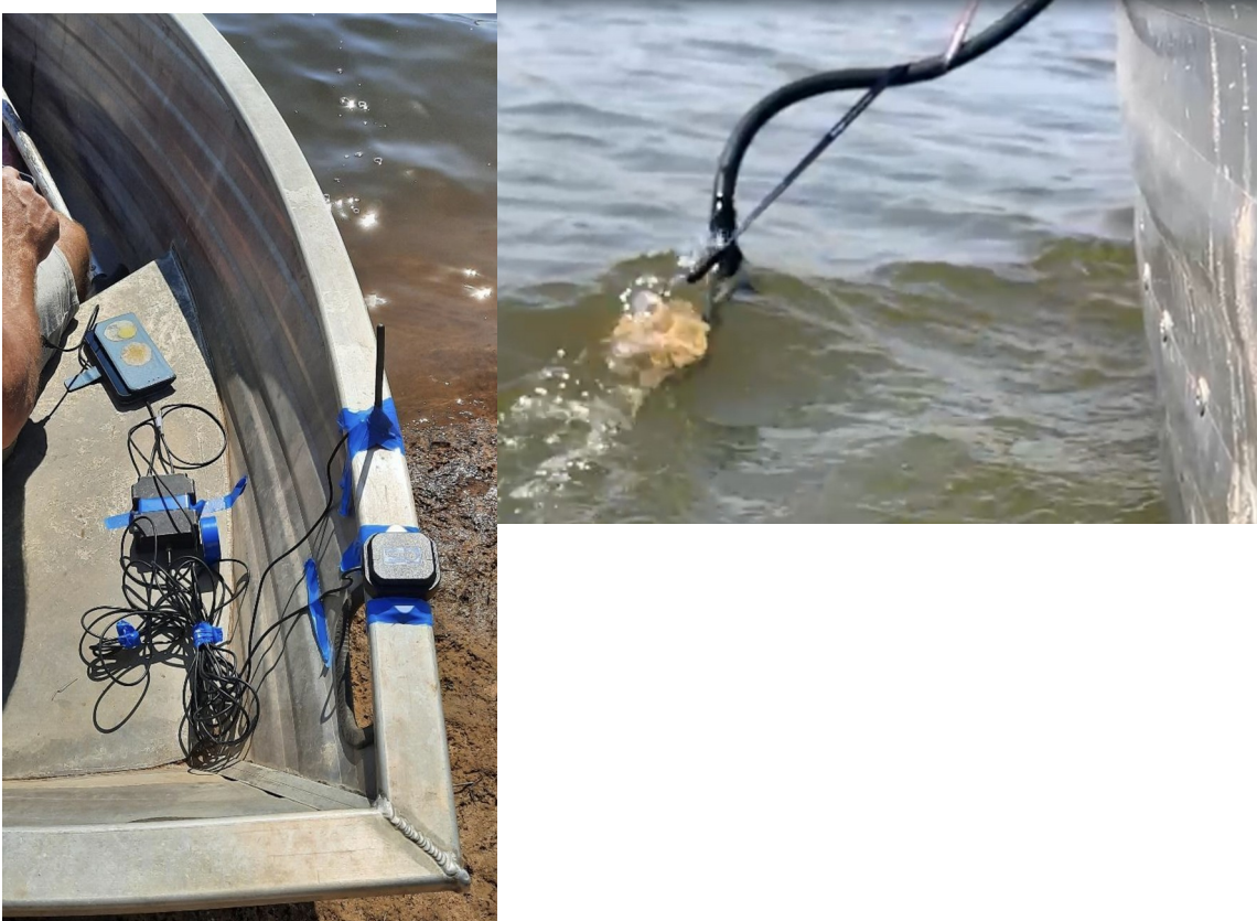
Figure 3.3: GNSS and fish finder set up on boat
