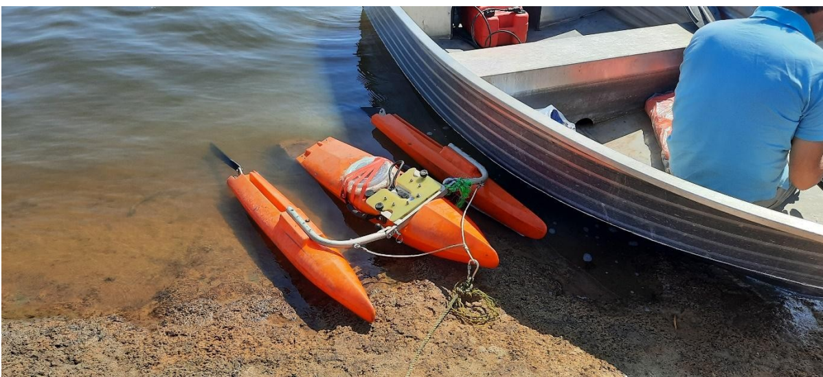
Figure 3.4: ADCP instrumentation side-by-side with fish finder set up for validation
