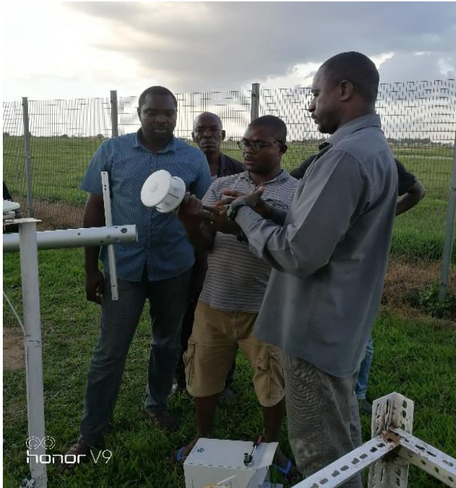
Coupling the Sensors' Component of one of the Installed AWOS by a Team of NiMet and WASCAL Personnel
